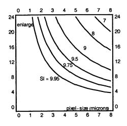
Figure 5. Sharpness as function of pixel-size and enlargement.
