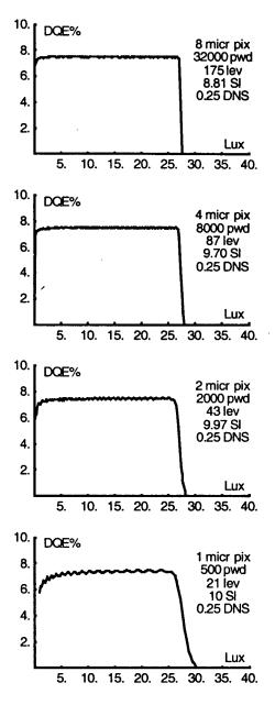
Figure 1. DQE-exposure curves for various pixel sizes
